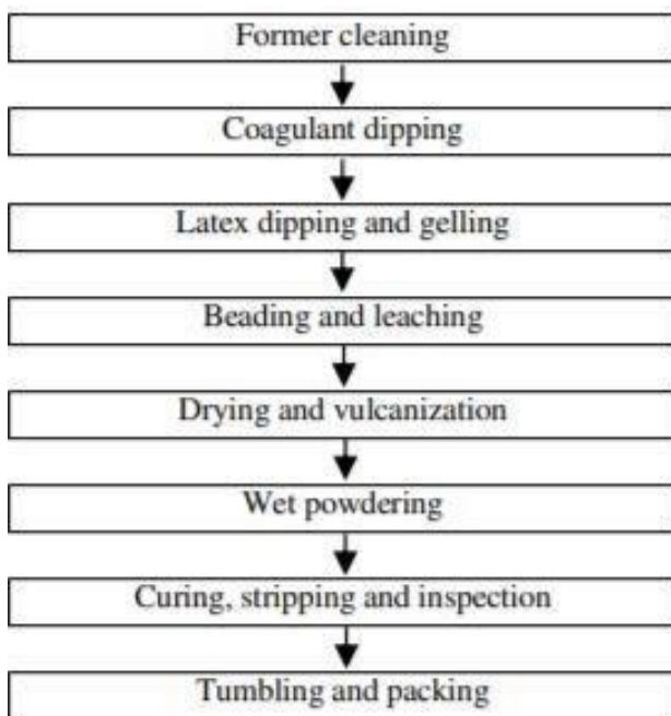
Fig. 1. General Glove Manufacturing Flow.
